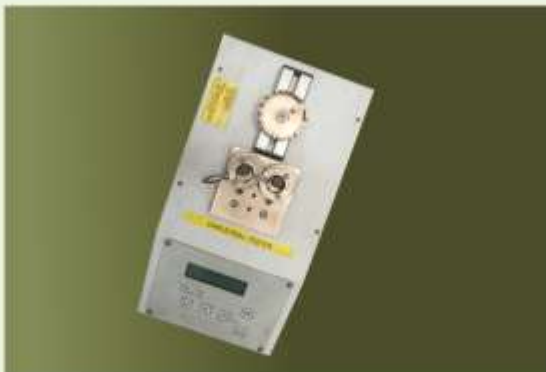
Cable Pullout Testing Machine
