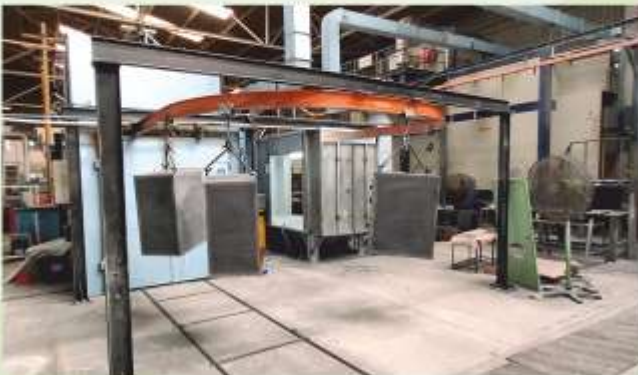
Powder Coating - Batch type Set-up
